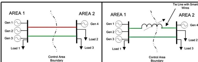
seeks to flow through that line in preference to the other (left part of the diagram). By installing PLGs on the upper line, impedance can be increased, balancing out power flows on the two lines (right part of the diagram) thus utilizing the total available transmission capacity.
