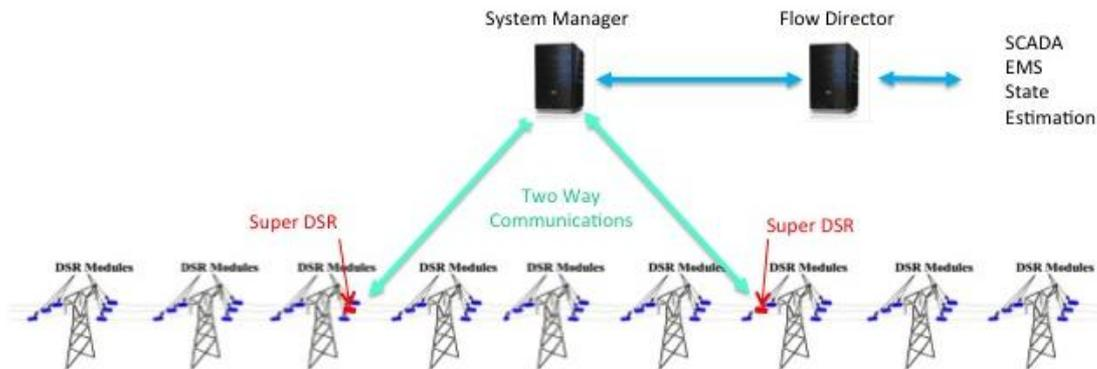
In addition to controlling PLGs, the communications capabilities allow PLGs to provide real time data on the lines including: line current, conductor temperature, frequency, sag and blowout angles, PLG status and PLG set point. Fault indication provides information of where a fault occurred (between which two PLGs). Other optional capabilities include conductor vibration and geomagnetic induced current detection.
